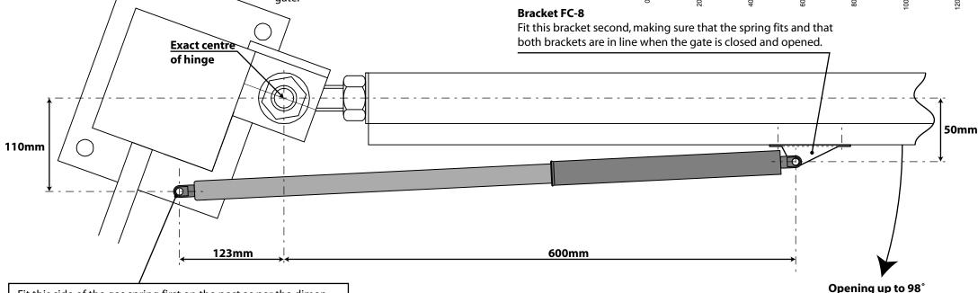
Fit this side of the gas spring first on the post as per the dimensions shown.
